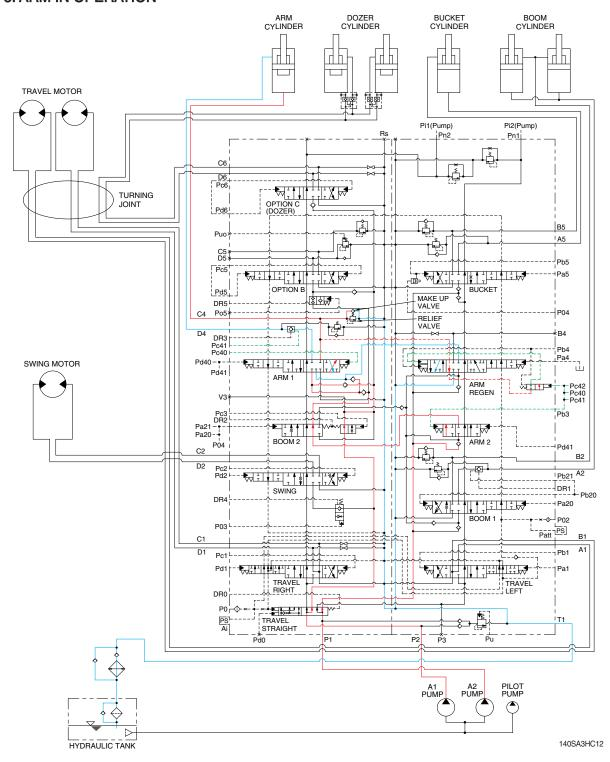
When the left control lever is pulled back, the arm spools in the main control valve are moved to the arm in position by the pilot oil pressure (Pc40, Pb3) from the remote control valve.
