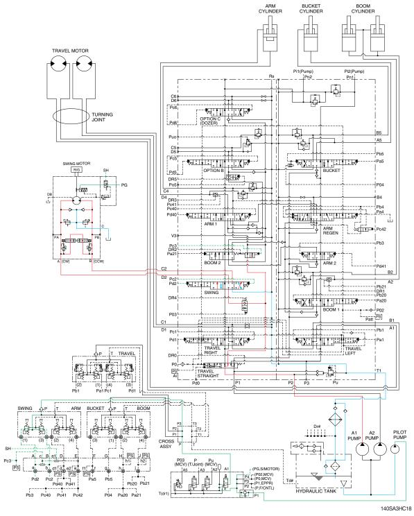
When the left control lever is pushed left or right, the swing spool in the main control valve is moved to the left or right swing position by the pilot oil pressure (Pc2, Pd2) from the remote control valve. Also the swing operation preference function is operated by the pilot pressure Pc3 (refer to page 3-14).
