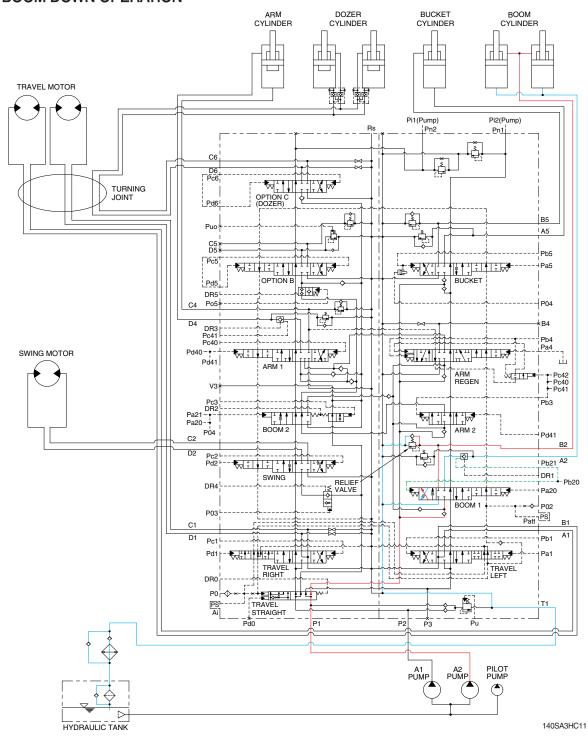
When the right control lever is pushed forward, the boom 1 spool in the main control valve is moved to the down position by the pilot oil pressure (Pb20) from the remote control valve.
